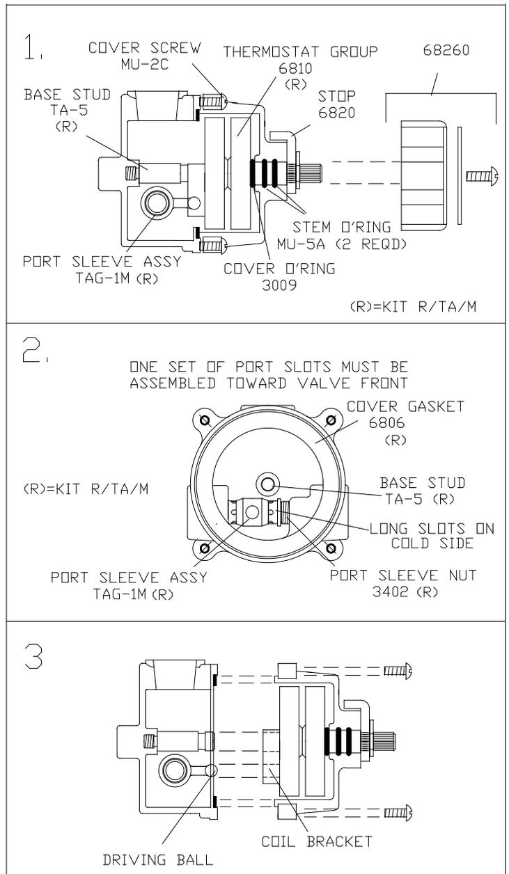
After installation, adjustment, and cleaning, always check the temperature of the valve when turned to full **HOT** per the warning on the front page, using a thermometer. Also check and if necessary adjust the temperature of the hot water source. **EXCESSIVELY HOT WATER (OVER 90°F) IS DANGEROUS AND MAY CAUSE SCALDING!!**
